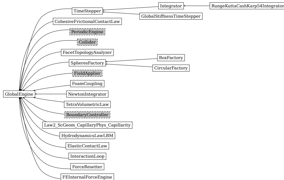
Fig. 25: Inheritance graph of GlobalEngine, gray dashed classes are discussed in their own sections: PeriodicEngine , Collider , FieldApplier , BoundaryController . See also: BoxFactory , CircularFactory , CohesiveFrictionalContactLaw , ElasticContactLaw , FEInternalForceEngine , FacetTopologyAnalyzer , FoamCoupling , ForceResetter , GlobalStiffnessTimeStepper , HydrodynamicsLawLBM , Integrator , InteractionLoop , Law2_ScGeom_CapillaryPhys_Capillarity , NewtonIntegrator , RungeKuttaCashKarp54Integrator , SpheresFactory , TetraVolumetricLaw , TimeStepper .
